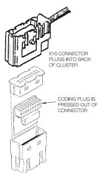
• Replacement coding plugs pre-coded by part number and are available from the parts department. Only order replacement instrument cluster coding plugs as indicated in *Parts Bulletin 62 01 02*.
